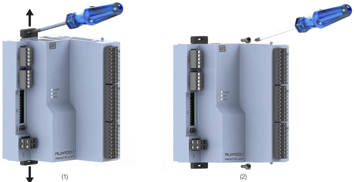
Figure 3.2: Mounting directly to the panel
